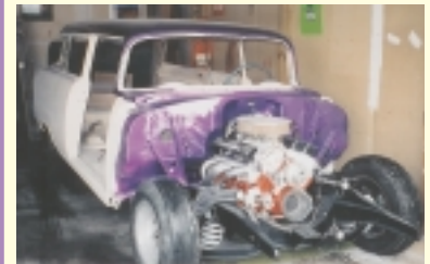
After white base coat, House of Kolor Passion Pearl (Purple) was applied to the firewall and roof.
