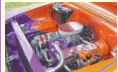
The power plant of this Handyman includes a 350 Chevy engine with a 700 R4 Transmission. Darney carries the flame details throughout the inner fender wells including the smooth custom radiator.
